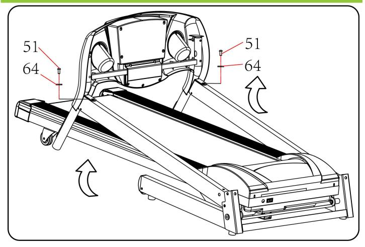
Hold the console frame, use the 5# Allen Wrench, lock the console frame onto left and right upright tube with bolt M8\*16(51)& lock washer (64) as the picture above
