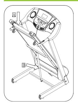
Support the position A, kick the position B by foot, and pull down the machine a little, the machine will fall down automatically. Please keep people and animal away to escape any hurt.
