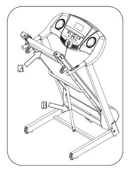
Hold the position A, pull up the machine, till cylinder gets the position B
