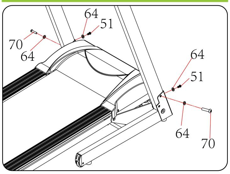
I. Use the 5# Allen wrench, drill through the Bolt M8\*45 (70) to Lock Washer (64), then lock the right upright onto base frame.
