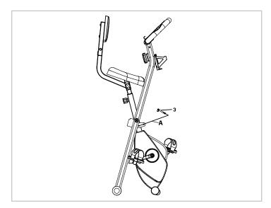
Using the Locking Pin (3) to fold and unfold the bike. When folded, the Locking Pin (3) is in Positon A.
