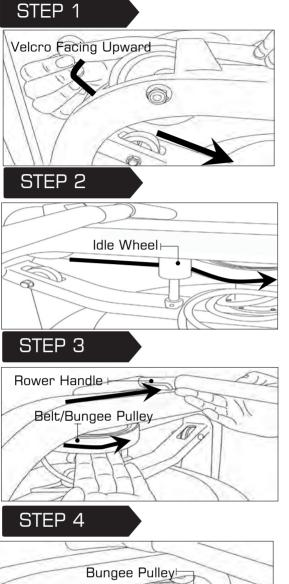
Begin reattaching the Rower Belt by threading around the Rower Belt Pulley with the Velcro side facing upward as illustrated.
