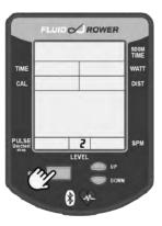
Turn handle to Level 2. Press Reset. Display will now show Level 3. Level 2 Calibration is complete.
