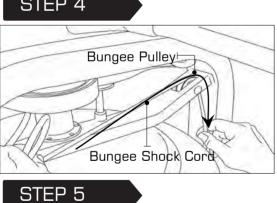
Rethread the Bungee Shock Cord (on opposite side of the Idle Wheel) back through the Bungee Pulleys and tie off at the Attachment Point.
