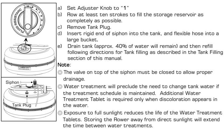
O Approximately 40% of tank water will remain. It is not possible to completely drain the A/R tank without disassembly.
