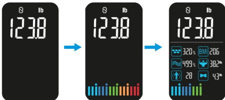
4. The scale will automatically shut down after displaying for about 15 seconds.
