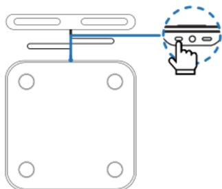
2. Charge the scale with a 5V/1A charger for about 2 hours.
