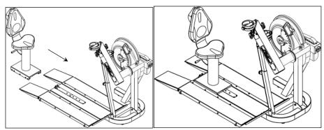
c) To remove the Seat: Lift and lower the Rear Safety lock, depress the Seat Lock Release Lever and slide the Seat rearward.
