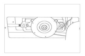
2. Using a long tool, push out the rear end cap as pictured below left. This will give you access to the tank
