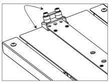
b) Seat Installation: Tilt the Seat slightly upward to allow the front Rollers to engage the channel. Then, lift the rear level and, while engaging the Seat Lock Release Lever, slide the seat onto the Baseplate as shown.
